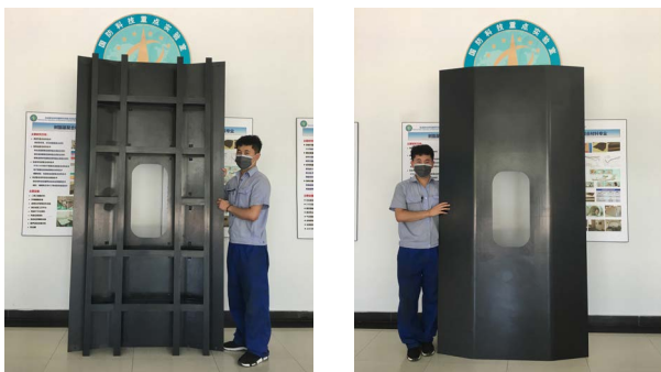
图 14 国内采用 SQRTM 成型工艺制备的纵横加筋壁板 Fig.14 Transverse and vertical stiffened panel manufactured by SQRTM in China
